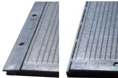
indented connecting bar engages flush with the surface and engages in the countersinks on the mat's edge → facilitates professional installation
