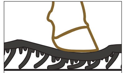
supporting studs have a cushioning effect at concentrating loads (when the cow gets up or lies down)
